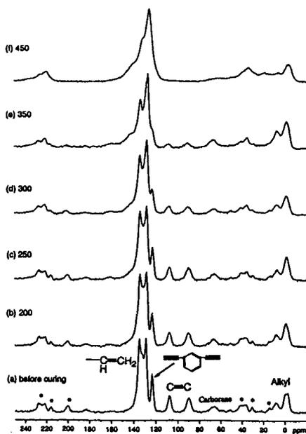
Fig.3  $^{13}\text{C}$  CP-MAS NMR spectra of silyl-carborane hybridized diethynylbenzene-silylene polymer cured at various temperatures: a) before curing; b) 200℃; c) 250℃; d) 300℃; e) 350℃; f) 450℃.
