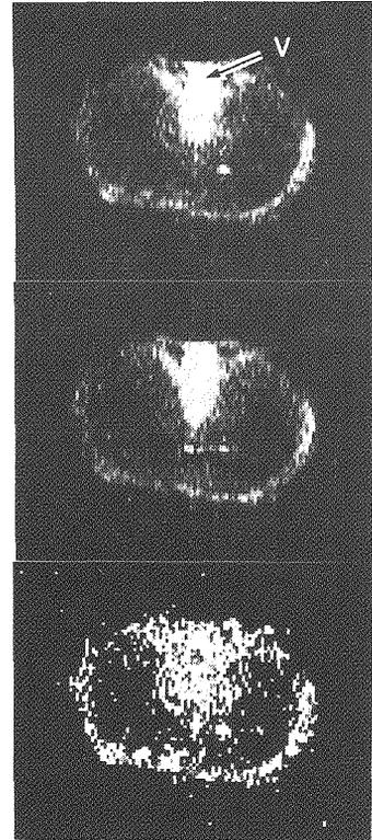
Fig. 2 An <sup>1</sup>H-NMR image (top), a diffusion weighted image (middle) and a diffusion coefficient image (bottom) of a 30 day old barley seed. The diffusion coefficient image was calculated by the formula of Stejskal-Tanner.
