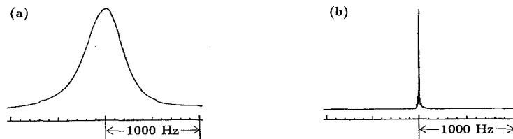
Figure 1. ^1\text{H} NMR spectra of water in Cd exchanged Y-zeolite (a) and liquid water (b) at room temperature.
