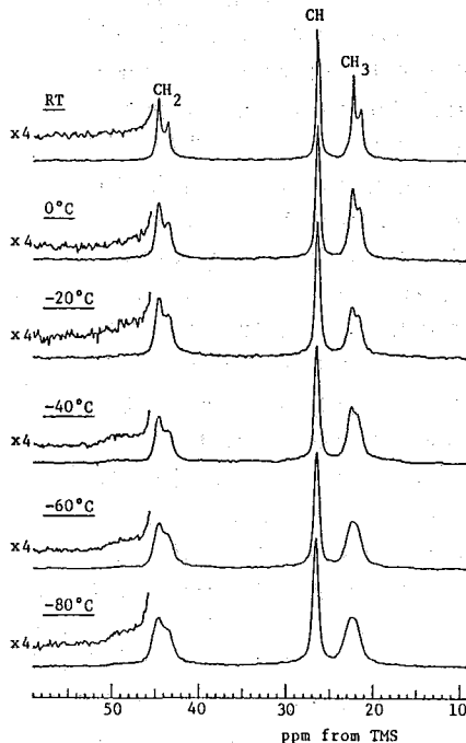
Fig. 4 CP/MAS 13 C NMR spectra of PP140 below room temperature
